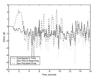
**Figure 3:** ERLE differences between methods 2–4 and the exact transform used in method 1, averaged over 100 ms blocks.
