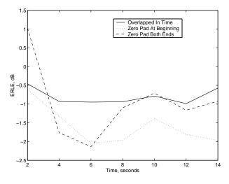
**Figure 5:** ERLE differences between methods 2–4 and the exact transform used in method 1, averaged over blocks of 2 s.
