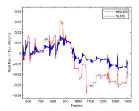
**Fig. 3**. Comparison of the real part of the first tap weight for the NLMS and MNLMS algorithms.
