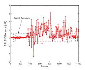
**Fig. 4**. ERLE difference between the proposed architecture and the conventional subband adaptive AEC algorithm on the AEC output in room noise.
