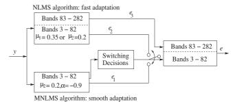
Fig. 1. Proposed dual-structured AEC architecture.
